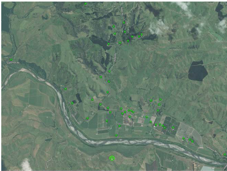
ePMP AP (bottom center) connects 33 subscribers in New Zealand
