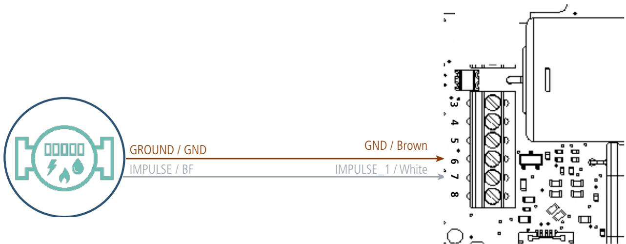
In this configuration, it is necessary to deactivate the input TAMPER of A-channel (register 320 bit 3 = 0) and preferably deactivate B-channel (register 320 bit 4=0) which is not used.
