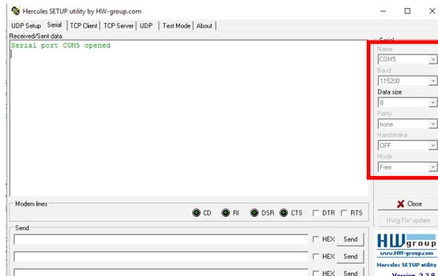
You must send a specific frame in order to move the device to configuration mode. Frame expressed in hexadecimals: 0x2B 0x2B 0x2B ou « +++ ».
