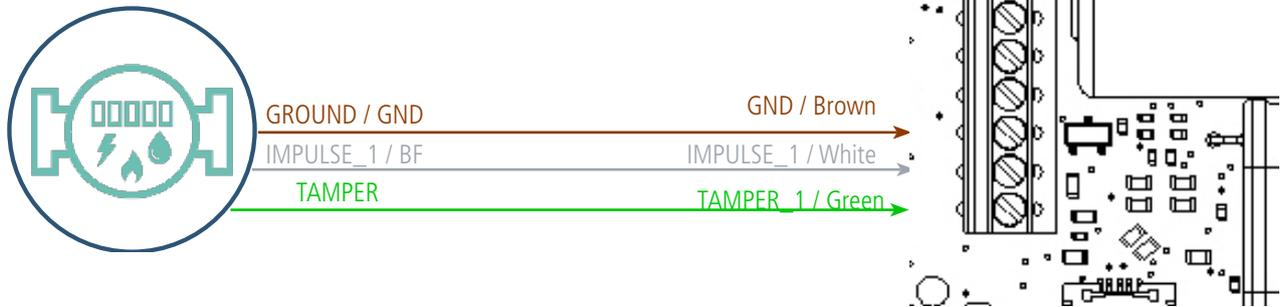
In this configuration, it is preferred to activate input TAMPER of A-channel (register 320 bit 3 = 1) and deactivate B-channel (register 320 bit 4=0) which is not used.
