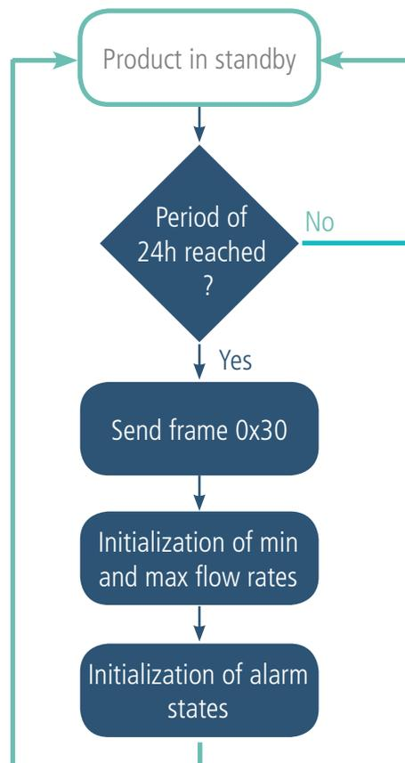
The transmission period of the daily frame is fixed (24 hours) and not configurable.
