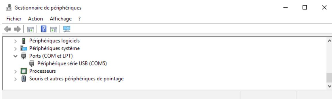
Using Windows: Verification that the device has been recognised to be functioning properly can be obtained by consulting the device manager. You should see the USB series device with a corresponding COM port number appear during connection.
