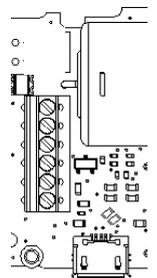
6 - Connect the ends of the meter cable to the screw terminals.
