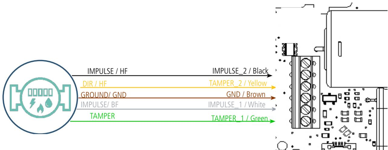
In this configuration, the 2 inputs (A & B) must be activated (register 320 bits 0 and 4 = 1). The combination of the pulse counts on channels A & B (IMPULSION\_1 & IMPULSION\_2) allows to know the quantities measured in the 2 directions. The activation of signals TAMPER\_1 & TAMPER\_2 (register 320 respectively bit 3 and 7 = 1) allows to generate alarms of tamper and wrong flow direction.
